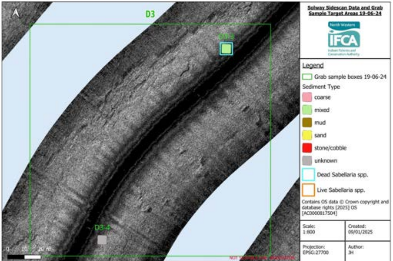
Figure 47 – Higher magnification of SSS data from target area D3 and grab sample contents for ground-truthing.
